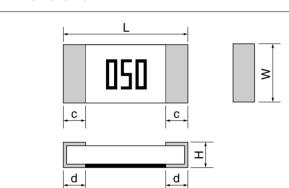
Resistance value is marking on surface. Please refer to Rated Resistance table on page 23. Please contact Kamaya Sales Dept. for marking of RCC16. RCC10 is no marking.
