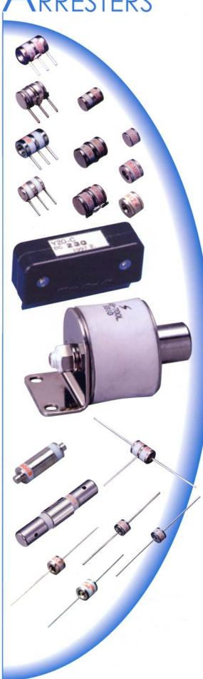
The Ceramic Gas Tube Arresters manufactured by Sankosha Corporation provide protection for personnel, equipment and circuitry from the abnormally high transient voltages which can be caused by lightning or electromagnetic induction. The arresters are designed with defined surge limiting characteristics. When the abnormal voltage on a line reaches that defined level, sparkover (or breakdown) occurs within the gas tube arrester, the surge is redirected and people and equipment are protected.
