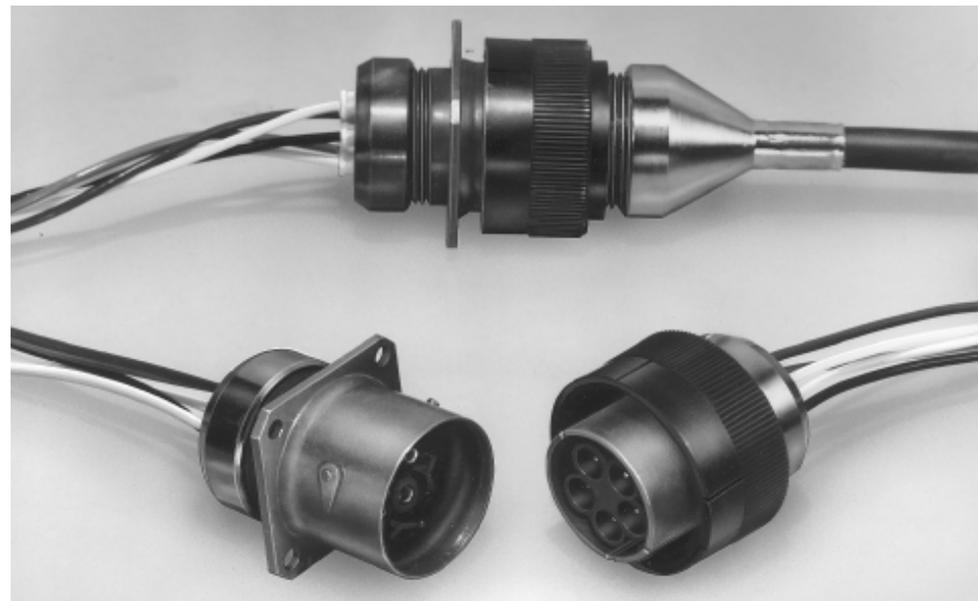
AMP 5-Pin Metal Shell Connectors are designed for high voltage circuits, especially in critical applications and harsh environments, such as shipboard applications. The connector is exceptionally lightweight and compact and can be used within a temperature range of -67°F to +257°F [-55°C to +125°C].
